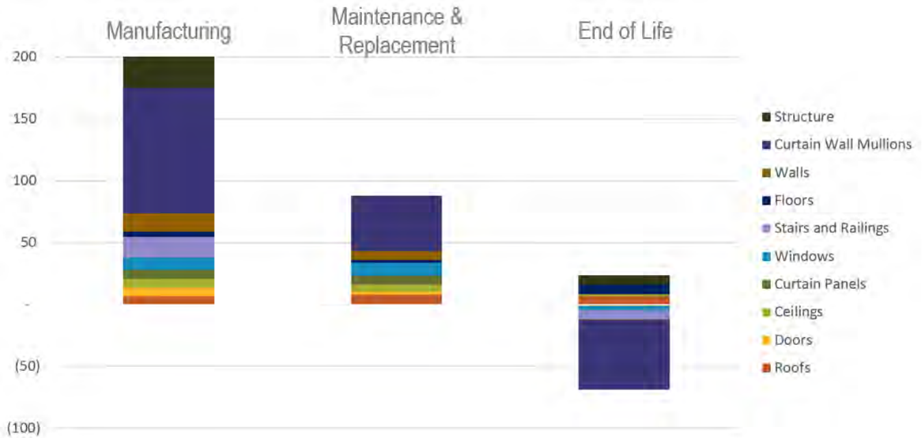
Figure 14. Total Scope 3 embodied carbon emissions (MTons CO 2e ) per Life Cycle Stage by Material Category
