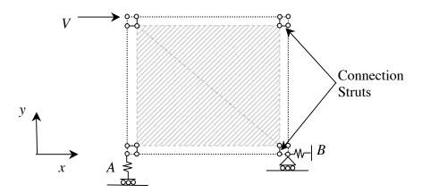
Figure 75: Schematic of Model of Test Developed for Linear Analysis Program
