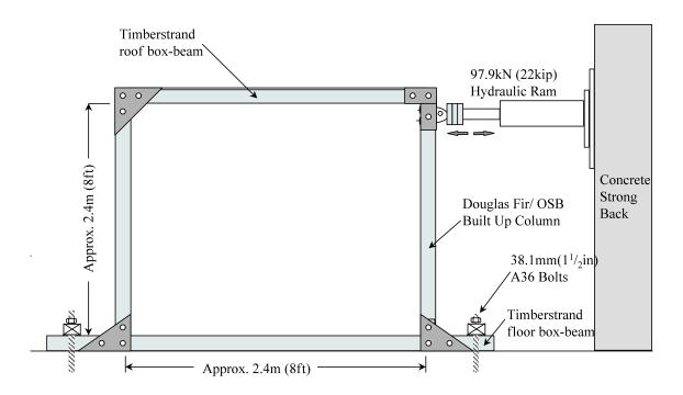
Figure 12: Schematic of Post and Beam Test Frame (Elevation)
