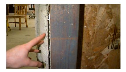
Figure 39: Facing Separation at +3% Drift
