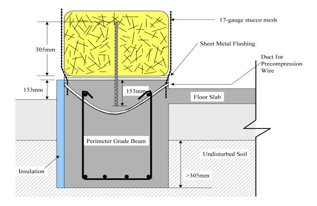
Figure 91: Foundation/Flooring System Cross-Section
