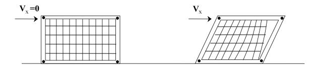
Figure 26: Predicted Behavior of Post and Beam Straw-Bale In-fill Wall w/out Facings, Subject to Monotonic In-plane Loading
