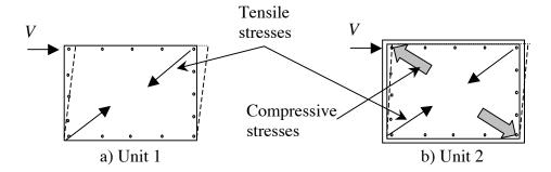
Figure 80: Deformations of Test Units
