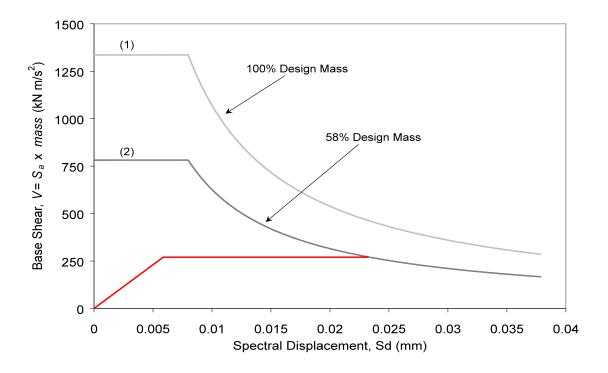
Figure 95: 10% Damped Base Shear Demand versus Spectral Displacement
