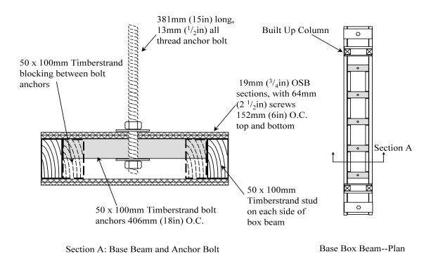
Figure 13: Cross-Section Schematic of Base Box Beam (1)
