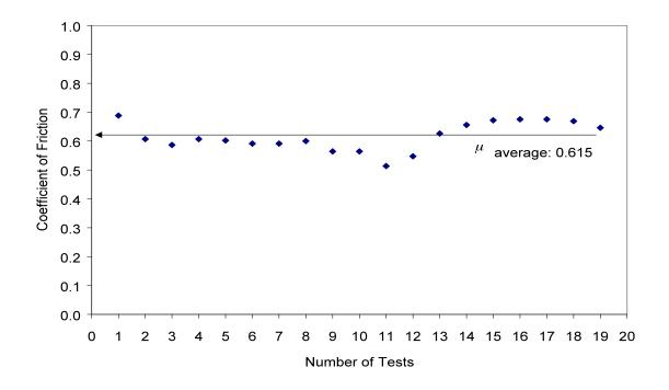
Figure 9: Scatter of Data Obtained from Coefficient of Friction Test
