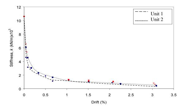
Figure 68: Stiffness Degradation for Units 1 and 2
