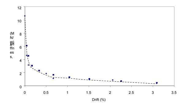
Figure 49: Stiffness Degradation, Test Unit 1
