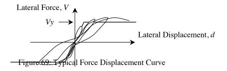
Since the shear modulus, G, times the width, w, of straw-bales is approximately 1/7 as stiff as the facings, then the facings are likely to carry the majority of the load at small drifts. It is assumed, probably conservatively, that the maximum strength may not exceed that predicted by ACI 318 (1995),  $V = 0.1667\sqrt{f'_c}b_w d$  (MPa) (equivalent to  $2\sqrt{f'_c}b_w d$  (psi) in English Units) for reinforced concrete members, due to the variability in stucco and plaster.
