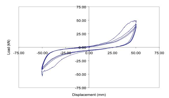
Figure 59: Hysteretic Load Displacement Loops for Test Unit 2 (±2% Drift)
