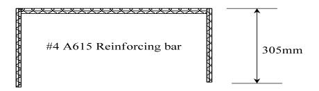
Figure 89: Staple for Corners in Straw-Bale Construction
