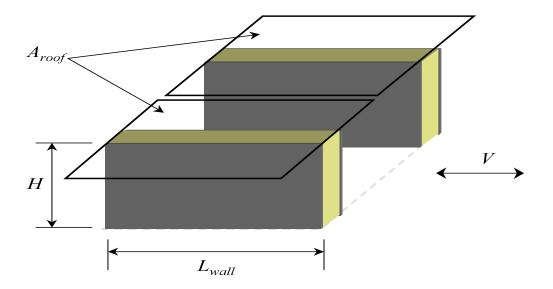
Figure 96: Schematic of Maximum Tributary Area per Horizontal Unit of Wall
