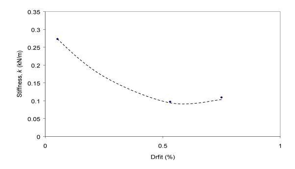
Figure 30: Stiffness Degradation Test Unit 0
