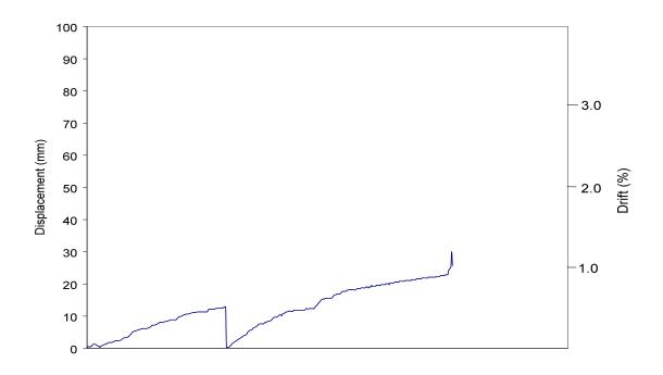
Figure 23: Monotonic In-plane Load Regime for Wall Unit 0 (Three-string bales, no facings)
