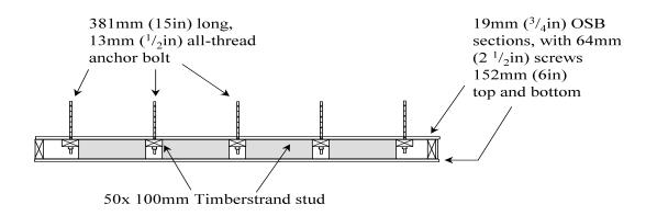
Figure 14: Cross-Section Schematic of Base Box Beam (2)
