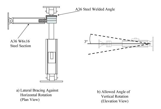
Figure 21: Lateral Bracing Against Horizontal Rotation and Allowed Angle of Rotation
