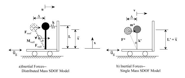
Figure 85: Inertial Forces Acting on Oscillators
