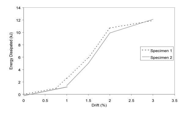
Figure 67: Energy Dissipation Capacity of Units 1 and 2
