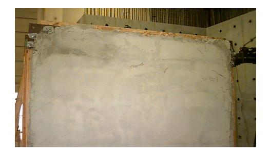
Figure 37: Damage to Stucco Facing, Test Unit 1, at ±1.5 to 2% Drift
