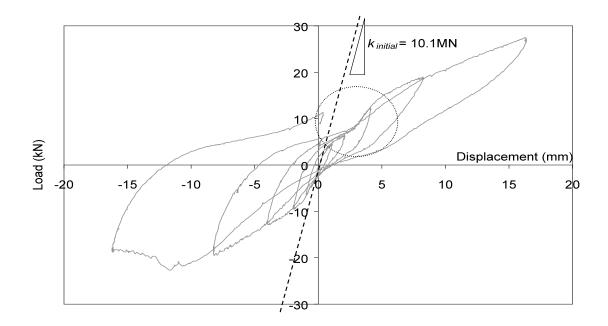
Figure 48: Initial Unit Stiffness, based on Force-Displacement Linear Relationship
