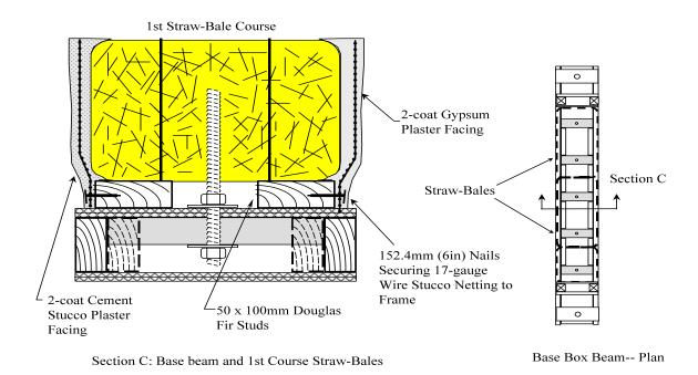
Figure 19: Typical Cross Section of Two String Straw-Bale Wall with Facings
