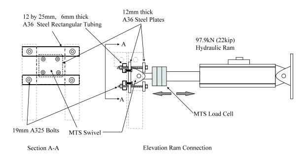
Figure 20: MTS Hydraulic Ram/Frame Attachment Schematic
