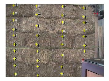
Figure 27: Observed Deformations at 2% Drift, Test Unit 0
