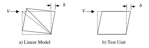
Figure 78: Schematic of Equal Force-Displacement Relationship between Model and Test Unit
