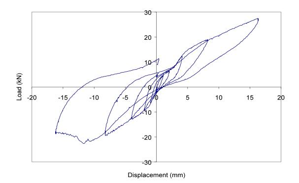
Figure 41: Hysteretic Load Displacement Loops for Test Unit 1 (±0.75% Drift)
