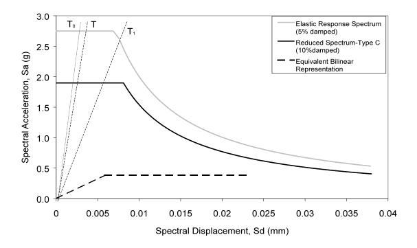
Figure 94: Acceleration-Displacement Response Spectrum (ADRS) for Model Structure
