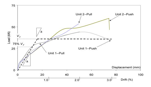
Figure 77: *Hy*, and *k*, as an Equivalent Bilinear Curve, and Envelope Curves for Test Units 1 and 2 versus Drift
