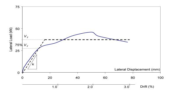
Figure 76: Schematic of Actual Load Curve and Linear Approximation
