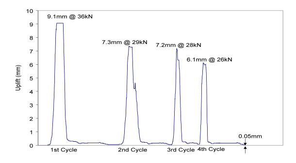
Figure 38: Uplift for Test Unit 1 at ±1.5 to 2% Drift
