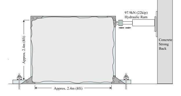
Figure 17: Elevation Schematic of Wall with Facings
