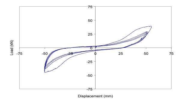
Figure 44: Hysteretic Load Displacement Loops for Test Unit 1 (±2% Drift)
