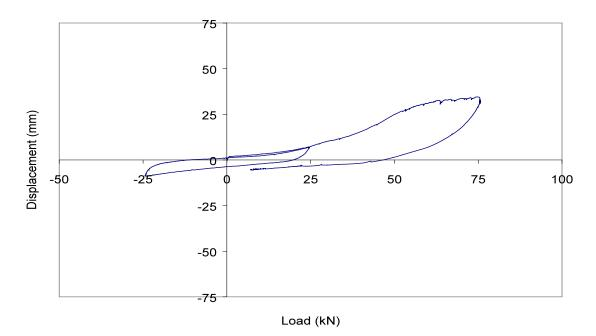
Figure 45: Hysteretic Load Displacement Loops for Test Unit 1 (+3% Drift)
