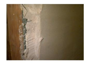
Figure 52: Damage to Plaster Facing, Test Unit 2, at ±1.5% Drift
