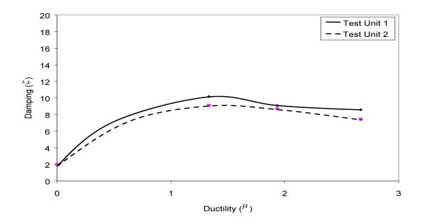
Figure 82: Equivalent Test Unit Damping Ratios,  $\xi$ , and Ductility,  $\mu$
