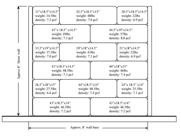
Figure 7: In-fill Wall Elevation Schematic (Two-string Bales)
