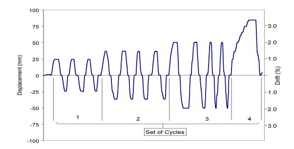
Figure 24: Cyclic Load In-plane Load Regime for Wall Unit 1 (Three-string bales, with plaster facings)
