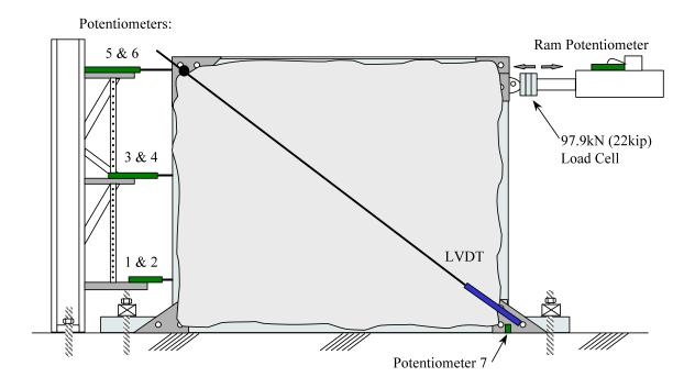
Figure 22: Wall Unit Instrumentation Setup
