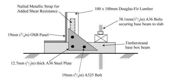
Figure 15: Detail of Seismic Connection for Base Box Beam and Built-Up Column
