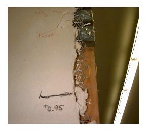
Figure 33: Damage to Test Unit 1 at ±1% Drift
