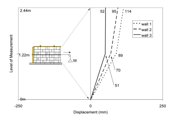
Figure 3: Graphical Representation of Deformation Induced by In-plane Loading on Load Bearing Straw-bale Walls w/out Facings
