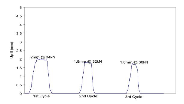
Figure 51: Uplift for Test Unit 1 at ±1.0% Drift
