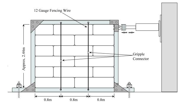
Figure 11: Schematic of Precompression Tie Wire Placement on Straw-Bale In-fill Wall
