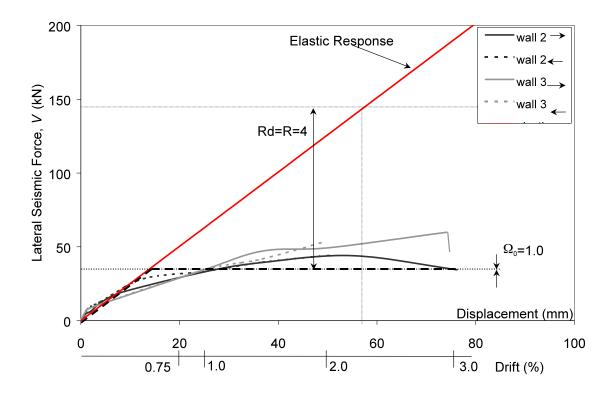
Figure 83: Elastic Response and Envelope Curves for Units 1 and 2 versus Drift
