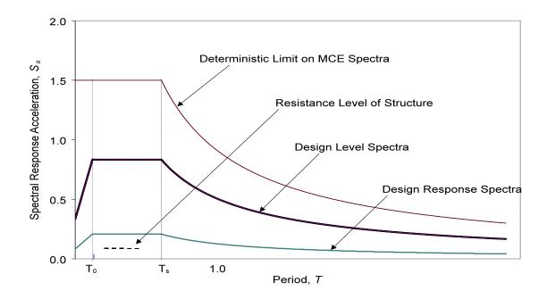
Figure 97: Reduction of Response Spectrum Calculated by NEHRP (1998)
