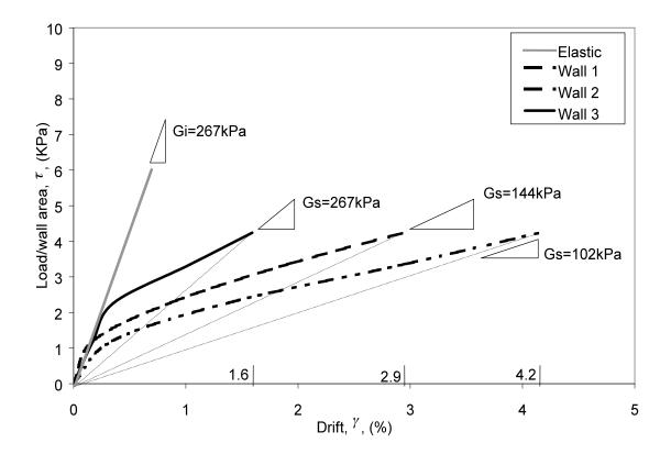
Figure 4: Lateral In-plane Monotonic Load per Area versus Drift
