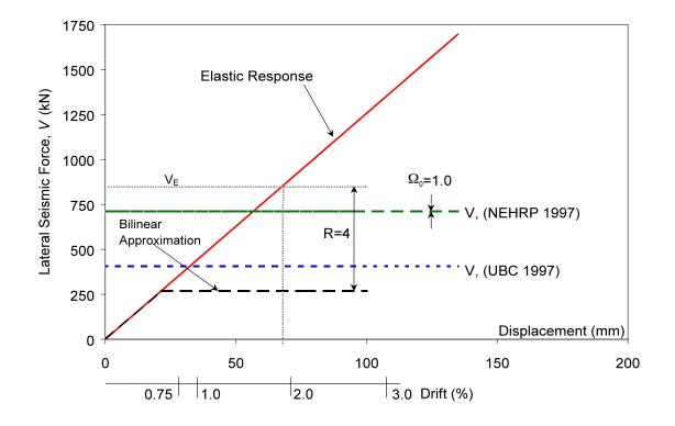
Figure 93: Expected Structural Envelope Curves and Calculated Base Shear Demand for Proposed Structure
