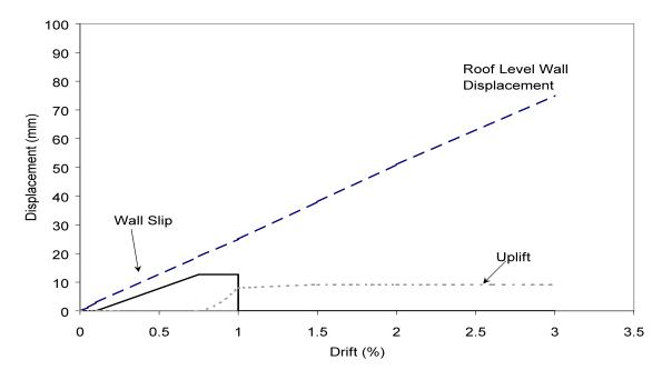
Figure 64: Uplift, Slip and Roof Level Displacement, Unit 1
