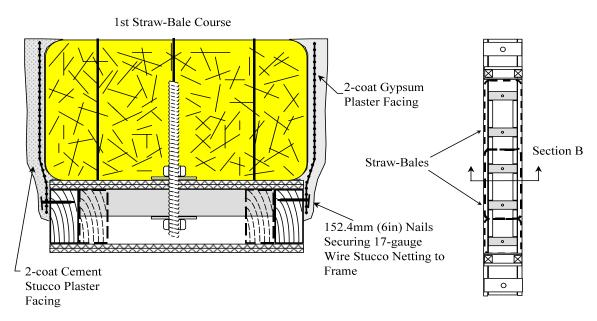
Section B: Base beam and 1st Course Straw-BalesBase Box Beam-- PlanFigure 18: Typical Cross Section of Three String Straw-Bale Wall with Facings
