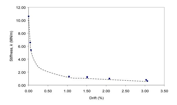
Figure 63: Stiffness Degradation, Test Unit 2
