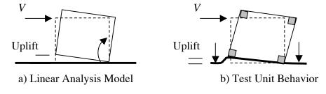
Figure 81: Comparison of Model Behavior vs. Observed Test Unit Behavior
