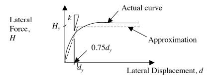
Figure 70: Schematic of Actual Load Curve and Bilinear Approximation
