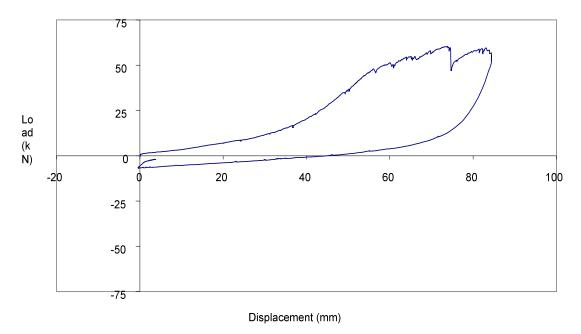
Figure 60: Hysteretic Load Displacement Loops for Test Unit 2 (+3% Drift)
