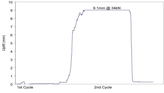
Figure 40: Uplift for Test Unit 1 at +3% Drift
