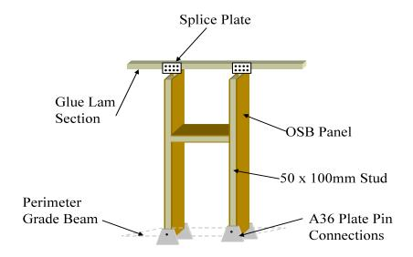
Figure 90: Post Framing Sections
