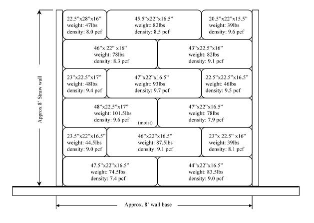
Figure 6: In-fill Wall Elevation Schematic (Three-string Bales)
