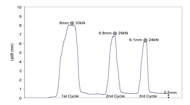
Figure 35: Uplift for Test Unit 1 at ±1% Drift
