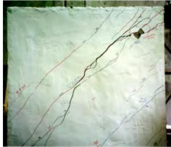
Figure 22: Failure of the Raap and Nichols wall in shear
