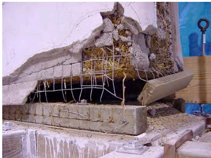
Figure 6: Flexural cracks in Wall E (2.5% drift level) Figure 7: Wall E mesh failure (7.5% drift level)
