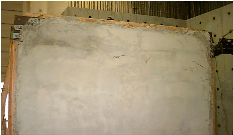
Figure 37: Damage to Stucco Facing, Test Unit 1, at  $\pm 1.5$  to 2% Drift
