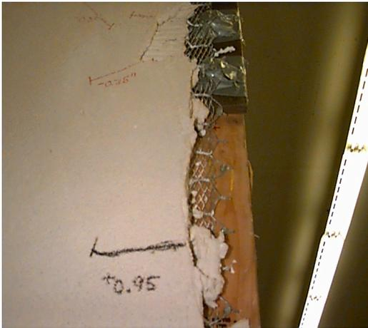
Figure 33: Damage to Test Unit 1 at  $\pm 1\%$  Drift
