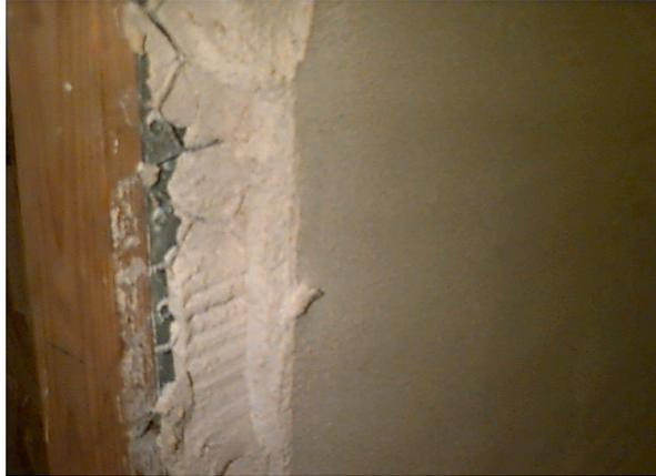
Figure 52: Damage to Plaster Facing, Test Unit 2, at  $\pm 1.5\%$  Drift
