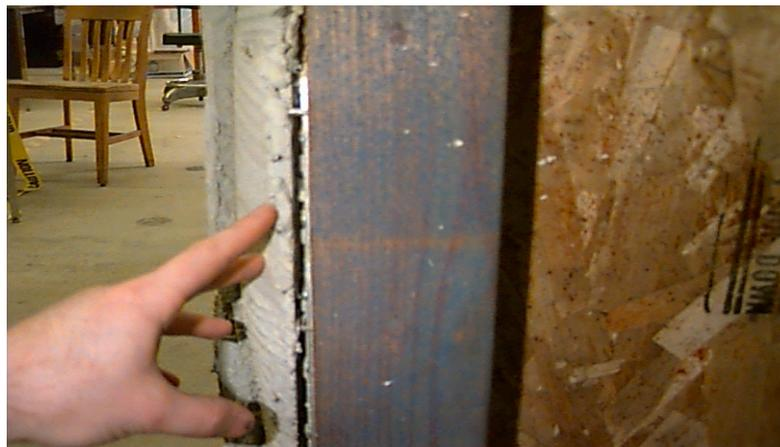
Figure 39: Facing Separation at +3% Drift
