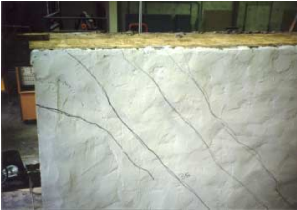
Figure 15a – Right face cracks during final test
