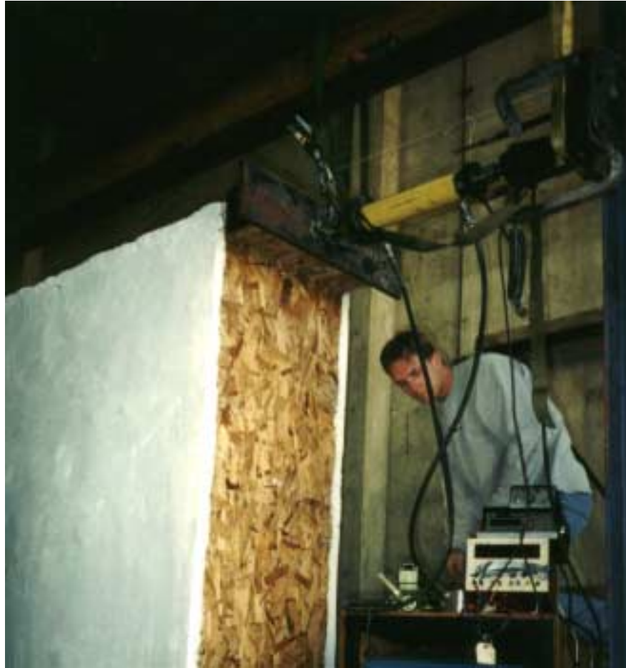
Figure 10 – Wall loaded during first test
